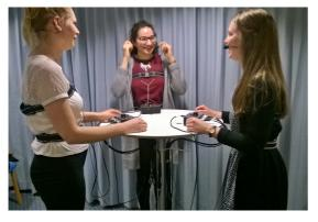
Figure 1. Students in the Phonetics Laboratory wearing transducer belts, each connected to a RespTrack, during a recording session.
